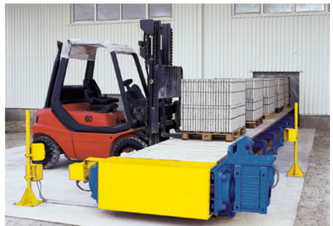
Slab package take-off station: Ready for transport.
