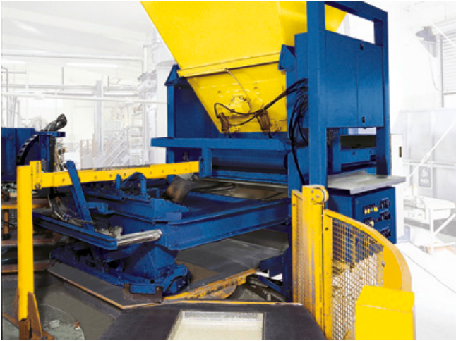
Back mix feeding device with feed box and belt feeder for exact slab thicknesses.
