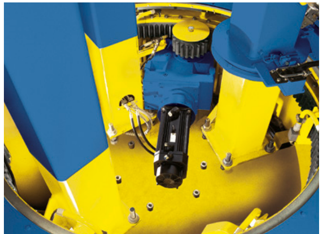
Servo turntable drive provides optimum acceleration and braking.
