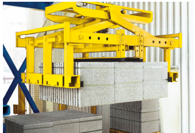
Slab package transfer device: Powerfully grabbed and gently placed.
