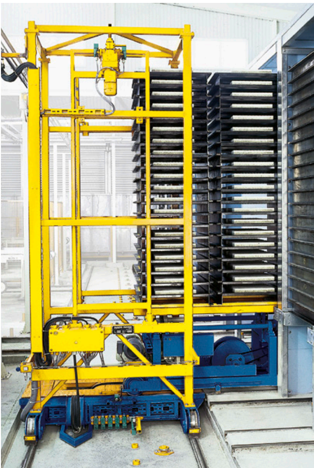
Racking system with programmed pallet stack transfer device.
